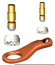
This cable lug is both PinBrazed to the cable and to the surface. No crimping tool is needed. The cable is inserted in the lug which is flatten and the cable is then PinBrazed to the lug by placing the brazing pin in the flattened hole.
